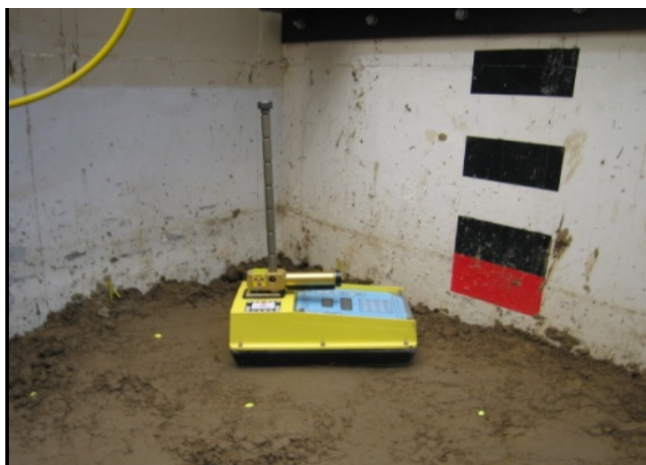
Figure 23: Nuclear density gauge device in use in test bed
