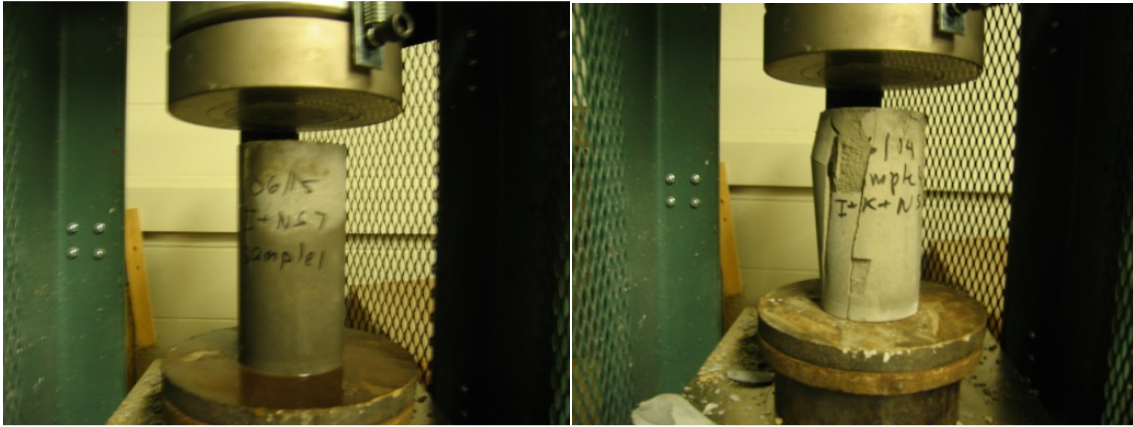
Figure 36: 28 day compressive strength test
