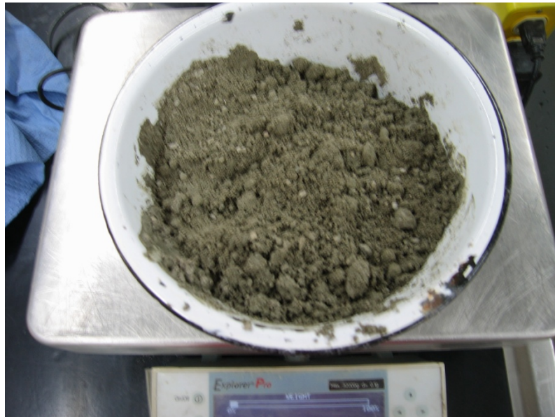
Figure 50: 1/10 th scaled aggregate pier material mixed with cement type I
