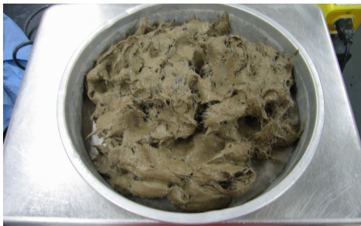
Figure 56: Loess + C(I) + fiber mix during sample preparation
