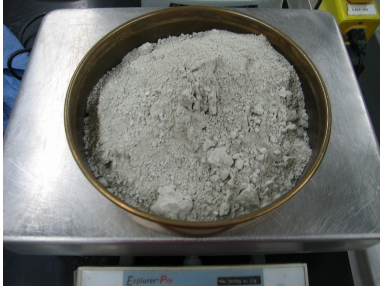
Figure 51: Cement type K compound
